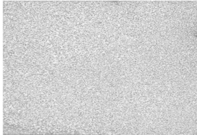
Figure 5.5 Uniform corrosion of Zinc exposed to hydrochloric acid
